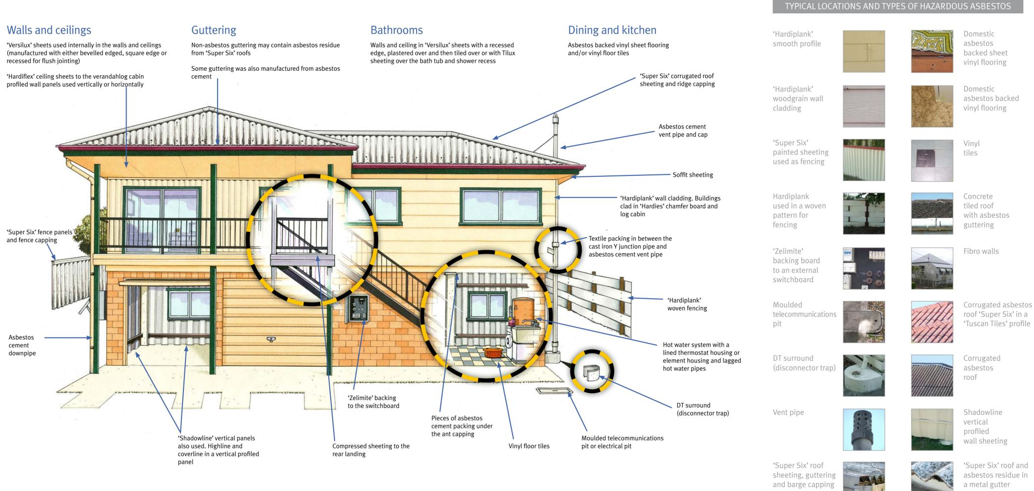
Buildings constructed after 1990 are unlikely to contain asbestos materials. The diagram shows areas where materials containing asbestos were commonly used during construction. These materials are not dangerous if they are in a good condition and remain undisturbed.
